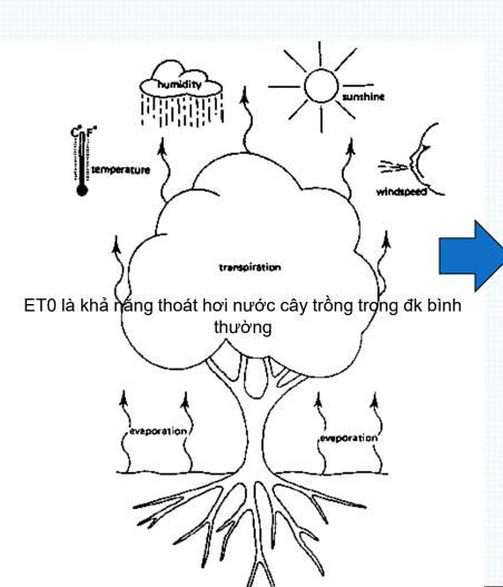
$ET_{0} = \frac{0.408\Delta(R_{n} - G) + \gamma \frac{900}{T + 273}u_{2}(e_{s} - e_{a})}{\Delta + \gamma(1 + 0.34u_{2})}$
