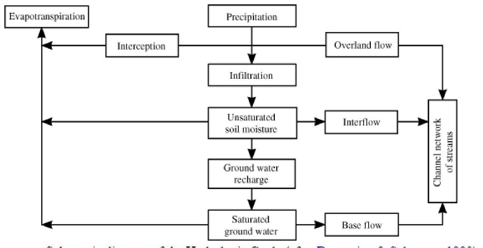
Schematic diagram of the Hydrologic Cycle (after Domenico & Schwartz, 1990)
