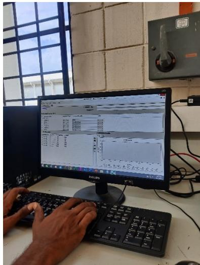
9. To obtain a positive value of 4cm, the test must be repeated, lowering the probe by 4cm (2 holes) and changing the "X-Offset" setting in the software to 40mm.
