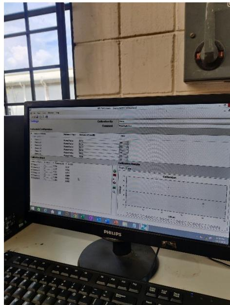
11. In the end, the calibration results will give a value in mm/V around 30-32mm/V.
