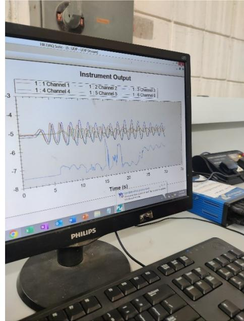
12. Save the analysis results and start the test with a frequency of 4.87Hz to obtain the wave amplitude variation over time.
