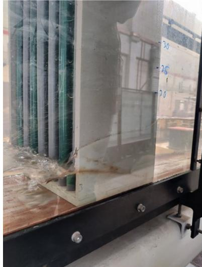
6. Evaluation of the percentage of probes submerged in water (approximately 30%)
