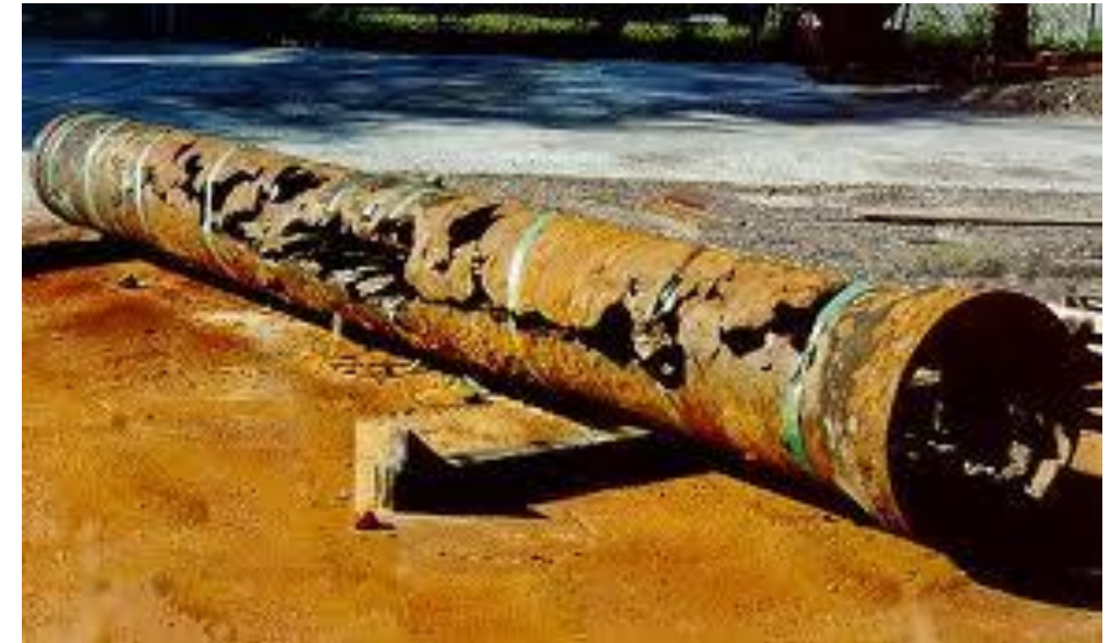
Corroded Carbon Steel Pipe!
