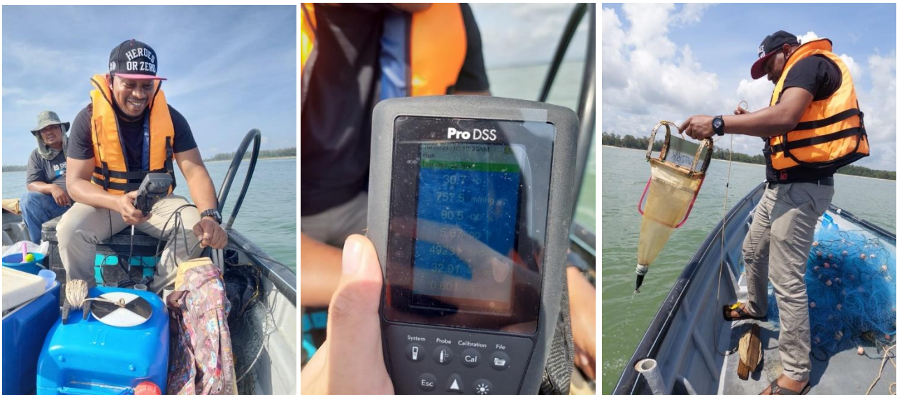
Figure 3 a, b & c: Sampling using the equipment. YSI Pro DSS Multiparameter Water Quality Checker Logger display. Sampling was also conducted for phytoplankton collection.
