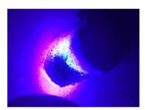
Detection of the tracer material in the field using a blue light / UV torch.
