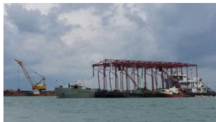
(a) Sand conveyer barge and pump vessel
